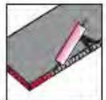
Coat cut edges with CP 606
