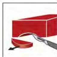
b) Cut blocks to size if cables are in place
