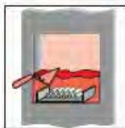
Put mortar into place
