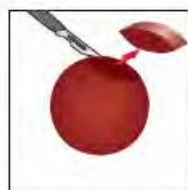
With cables, cut plugs to fit around cables
