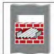
Build up blocks to fill the opening
