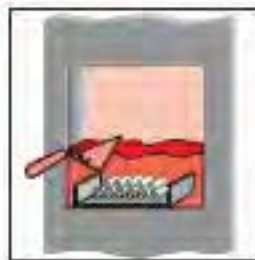
Put mortar into place
