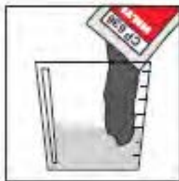
Mix CP 638 mortar (by adding mortar to water)
