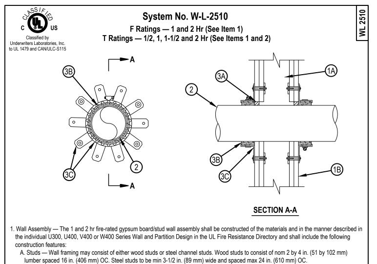
B. Gypsum Board\* — The gypsum board type, thickness, number of layers, fastener type and sheet orientation shall be as specified in the individual Wall and Partition Design in the UL Fire Resistance Directory. Max diam of opening is 9 in. (229 mm).
