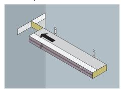
Coat back of intumescent facing strip with CP 606/CFS-S ACR. Take section of CP 674 barrier for other wall face and position end to the intumescent strip from previous step.
