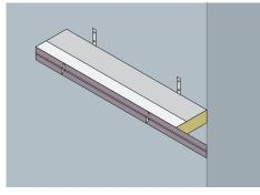
Fit CP 674 to extend past the corner by the width of the CP 674 barrier. Remove section of mineral wool from CP 674 back to corner leaving intumescent strip.
