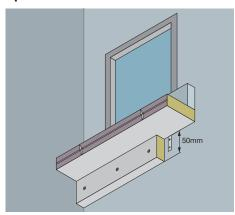
Where access constraints mean brackets cannot be fixed above the cavity barrier, the brackets may be fixed beneath the barrier, with 50 mm CP 670 (coated board) used to protect brackets.
